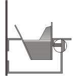
Adjust the burn grate top so that the burn grate top sits firmly on the top of the burn box and level.
